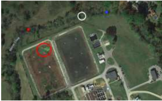
Figure 24: Google Earth image of waste treatment plant between two measurement points on Beaver Creek. The downstream point (red dot) is out of compliance whereas the upstream point (blue dot) complies with Phosphorus requirements. The waste treatment plant outfall (white circle) may release emissions from a potential algal growth in the treatment plant (red circle).
